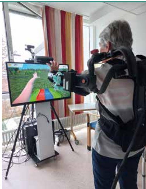
Figure 1. Upper limb rehabilitation after stroke delivered by a hybrid neuroprosthesis with proximal support by FES plus robotics and distal support by FES alone. This hybrid device has been developed within the ReHyb project and is currently tested for feasibility. Informed consent was collected to publish the picture
