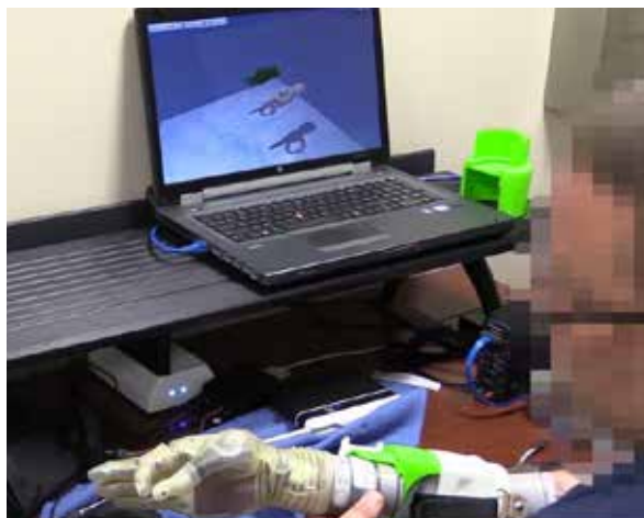
Fig. 2: Subject P1 using a virtual environment to replicate random finger movements with the prosthetic arm
